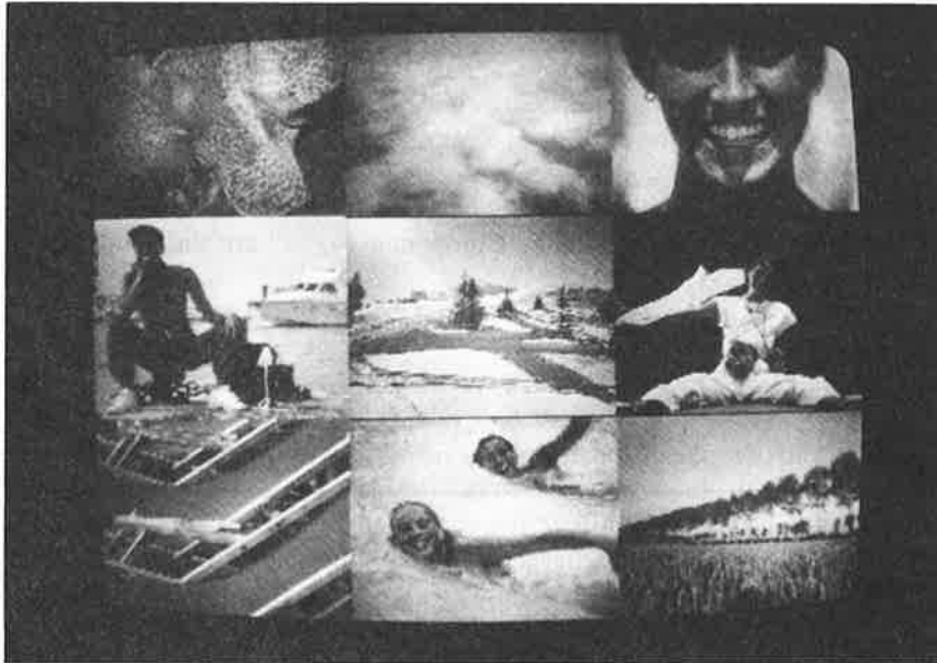
FIGURE 12.23 The use of field memories also makes it possible to combine parts of pictures. The example given here is 'multi-picture-in-picture', where the signals originating from several different transmitters are displayed simultaneously. This can be a very useful facility when making a selection from a large number of programmes.
